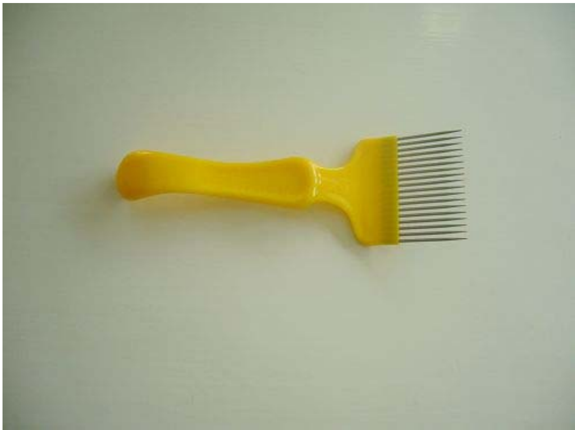
Uncapping forks(straight,with stainless steel needles)
